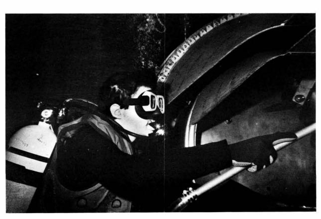
IN-DEPTH TECHNOLOGY — Richard Cleary of K-Tech and his SCUBA gear remove bubbles from the transition section of a PBFA-II module now being tested in the Demon facility in Area IV. (Underwater photography by Mike Eaton, K-Tech)
